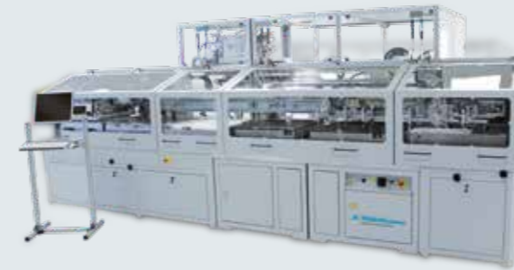
MTT 2462 A Wire Embedding and RFID Inlay Production System
